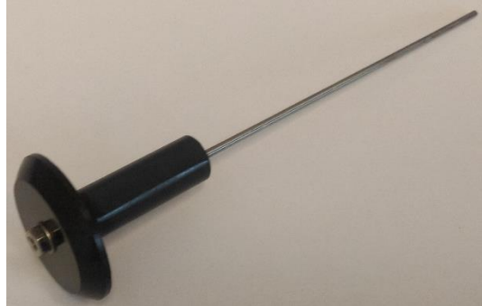
Figure 2: Valve body with attached LVDT armature
